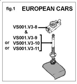
VS001.V3-9 = Ø 50mm VS001.V3-10 = Ø 35mm VS001.V3-11 = Ø 27mm
