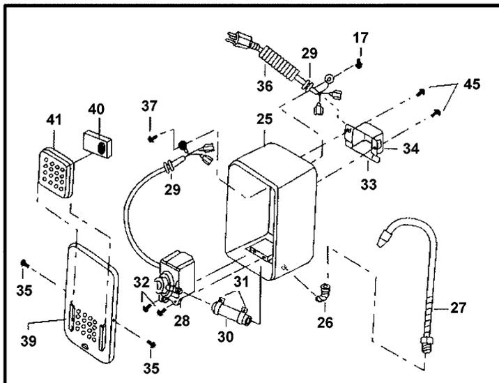
Exploded view of the pump assembly
