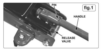
as shown in fig.2 and open the valve by turning the handle anti-clockwise, place the handle back into the jacking socket and pump for 30 to 40 seconds. When complete, close the release valve by turning the valve nut clockwise.
