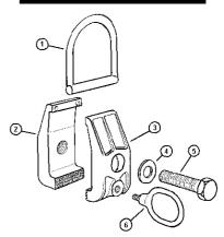
Item Part No. Description Item Part No. Description 184.D6020700 184.C0006515 Plain Washer, D14 Stirrup 184.D6001400 Jaw, Threaded 184.C0000130 Screw, M14x50 184.D6001500 Jaw, Plain 184.D2510600 Pull Ring
