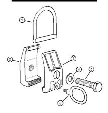
Item Part No. Description Item Part No. Description Stirrup 184.D6020700 184.C0006515 Plain Washer, D14 5 184.D6001400 Jaw. Threaded 184.C0000130 Screw, M14x50 184.D6001500 Jaw, Plain 184.D2510600
