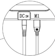
Connect the switch cable to the DC port
