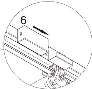
Insert the adaptor (6) to the bracket of the tabletop
