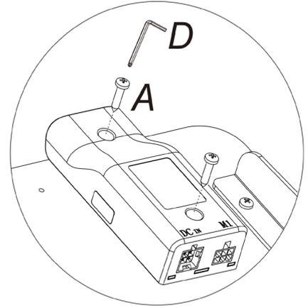
Fix the hand switch with the screw (A) and tighten it with 5\*5 wrench (D)
