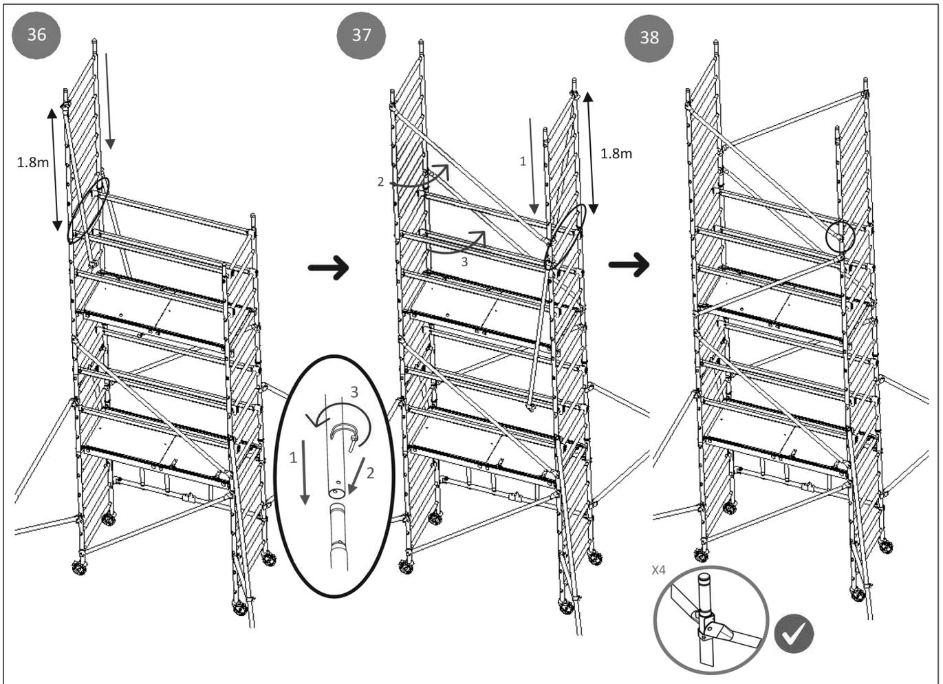
**Move the 1st platform to the 20th rung, refer to step 17, along with the rails, step 20, put in the toeboards step 23**
