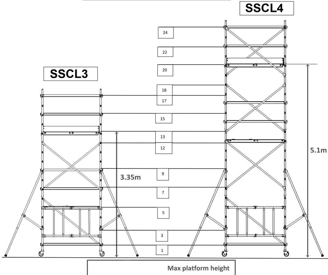
Platform height  $\neq$  working height - Adapt the platform height to the working area
