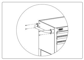
Fit side handle at swivelling castor end. Attach with 4 M6x16mm screws, tighten with hex key.
