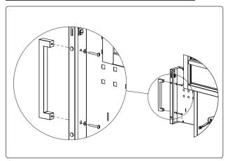
Fit handles to doors, use M4x30mm screws
