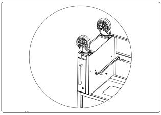
Position slider up to holes on inside panel. Attach with M6x12mm screws, tighten with screwdriver and hex key.
