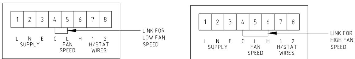
Before the unit will switch on it must have a low voltage humidistat wired into it with the NC contacts wired to the terminal block inside the electrical box as shown below.
