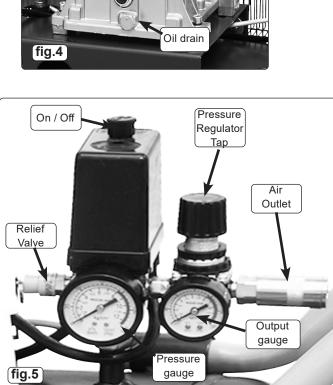
Dil Sight Glass the tank rises and that the compressor stops automatically when the maximum pressure value allowed - written on the plate and shown on the gauge (fig.5), is achieved. The compressor will now operate automatically. The pressure switch stops the motor when the maximum tank pressure is reached and restarts it when the pressure falls below the minimum threshold - approx. 2 bar (29psi) less than the maximum pressure.
