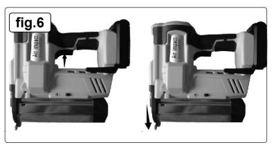
Squeeze the trigger, keep squeezing and don't release.
