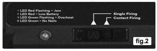
LED RED flashing: Jam LED RED: Low battery
