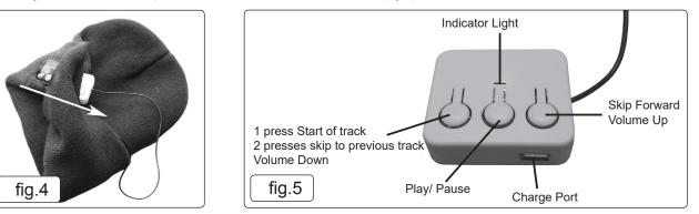
4.4.2. Using a mains adaptor or laptop charge the device. The indicator light will shine red while the device is charging (fig.5).
