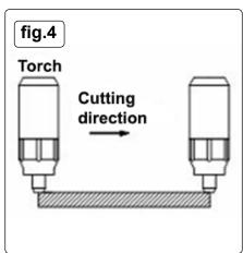
Keep a space between the nozzle and the workpiece. Pressing the nozzle on the workpiece could cause the nozzle to stick, reducing the smoothness of the cutting action.
