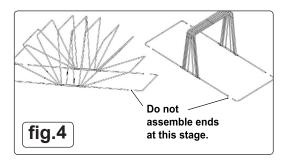
4.2.4. Ensuring that the correct side of the cover is facing outward, thread the end members into the cover sleeve and also engaging the ground fixing tab (item J) (fig.6.). Draw the cover over the remaining spars and fix in place using the hook and loop tabs built into it.
