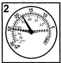
**READING:** When the throttle is suddenly opened then released the needle should drop to below 5inHg then bounce up to approx. 25in Hg settling back to original reading.
