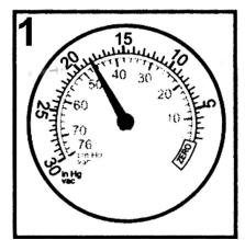
READING: 16-21 in Hg with needle
