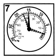
READING: Readings slightly lower than for lower for normal engine including when throttle is suddenly opened then released.
