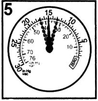
**READING: Reading slightly low and** fluctuating slowly. CAUSE: Over lean or rich mixture. Check and reset in accordance with
