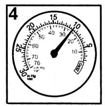
READING: Reading low but steady. CAUSE: Retarded ignition timing. Confirm using timing light and reset to manufacturer's specification.
