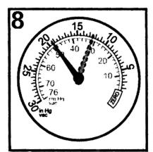
READING: Regular drop between normal and low reading.
