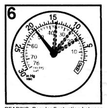
**READING: Regular fluctuation between** normal and low readings. CAUSE: Blown cylinder head gasket between two adjacent cylinders. Carry
