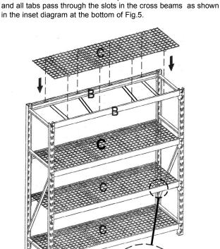
4.6 See Fig.5. Each wire deck 'C' is reinforced with four cross
