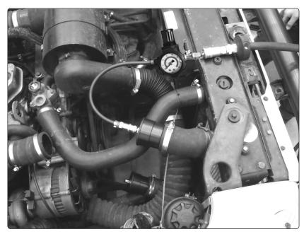
Example (left) shows the kit testing a turbo system intercooler for integrity.
