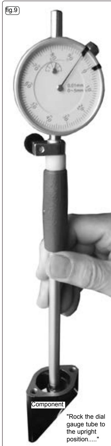
"Offer the anvil end into the bore slightly tilted...."
