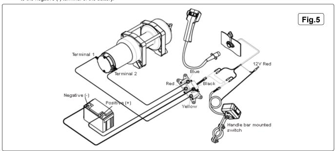
3.2.3 Connect the yellow wire to the positive terminal of the winch, marked as (1) on the rear of the motor case, and to the yellow marked terminal of the relay block. Connect the blue wire to the negative terminal on the winch, marked as (2), to the blue terminal on the relay block. See fig.5.
