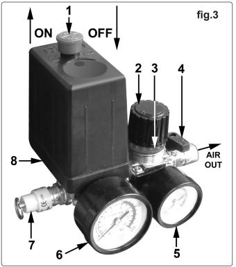
b)The main gauge (fig.3.6) indicates the pressure inside the main tank, **NOT** the pressure supplied to the air equipment, which is shown on the smaller gauge (fig.3.5). Should the pressure in the main tank exceed the pre-set switch (fig.3.8) maximum, the safety valve (fig.3.7) will activate. **WARNING! For this reason DO NOT tamper with, or adjust, the switch or the safety valve.**
