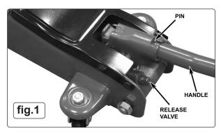
as shown in fig.2 and open the valve by turning the handle anti-clockwise, place the handle back into the jacking socket and pump for 30 to 40 seconds. When complete, close the release valve by turning the valve nut clockwise.
