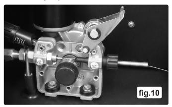
6.1.2 The roller groove size is stamped on the face of each roller adjacent to the appropriate groove. Ensure that the groove size you require is positioned furthest away from you so that it will be in line with the wire feed path.
