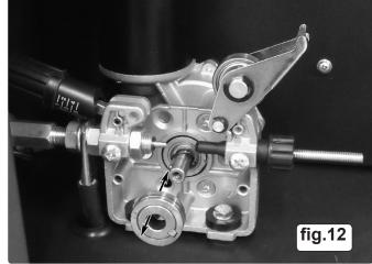
6.1.5 Once the carrier is free from the main drive, you can now slide the roller off the carrier as shown below in fig.13A. Take care not to unseat the loose key that aligns the roller with the carrier. The roller can now be reversed or replaced as required. In either instance the required drive groove must be furthest away from you at the back of the roller in order to align with the wire drive path.
