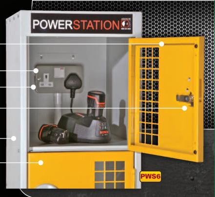
Battery charging locker bank, designed to charge power tool batteries, and mobile phones whilst keeping them safe & secure – ideal for the site office. Six separate compartments, each containing double sockets connected in series to a 230V RCD protected plug. Doors fitted with cam locks and perforated for ventilation. Lockers finished in an anti-bacterial epoxy powder coat. Each lock is serial numbered for replacement keys.
