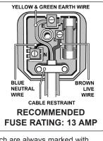
Double insulated products, which are always marked with this symbol, are fitted with live (brown) and neutral (blue) wires only. To rewire, connect the wires as indicated in
